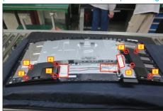
Disconnect the lamp cable, speakers' cable, LED cable, FFC cable from the connectors of the board. Use a Philips-head screwdriver to remove 4pcs screw for unlocking the USB unit, then disconnect the eDP cable away from board and release the USB unit from the hooks of the middle frame.
