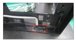
Tear off 2pcs shading tapes and 1pcs acetate tape, and then disconnect the panel lamp cable from the two connectors of the panel module.
