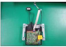
Release the two speakers from the probers of the middle frame and put it aside. Use a Philips-head screwdriver to remove 21pcs screws for unlocking the middle frame with the panel module.
