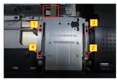
Use a Philips-head screwdriver to remove 1pcs screw for releasing the USB unit, then remove the USB cover, then use a Philips-head screwdriver to remove 1pcs screw for locking the USB board. Disconnect the USB connective cable.
