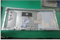
Remove the circuit boards from the bracket chassis module, and then disconnect all of the cables. Use a Philips-head screwdriver to remove 3pcs screws for unlocking TBT board with interface board.
