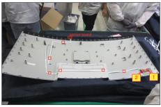
Use a Philips-head screwdriver to remove 2pcs screws for unlocking the IO cover with bracket, then release the IO cover away from the main bracket chassis.
