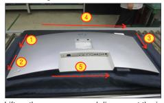
S6 Lift up the rear cover, and disconnect the joystick cable and sensor cable away from the connectors, and then remove the rear cover and put it aside.
